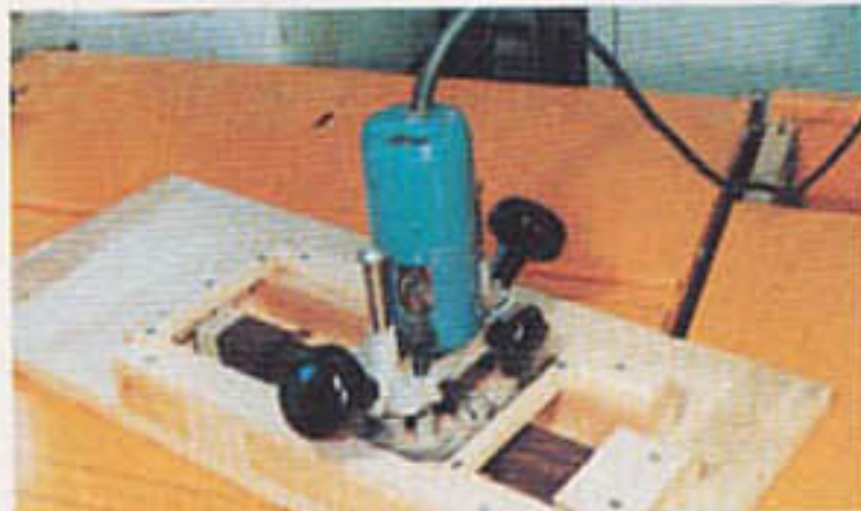
Homemade routing jig makes the flutes for the cabinet columns
