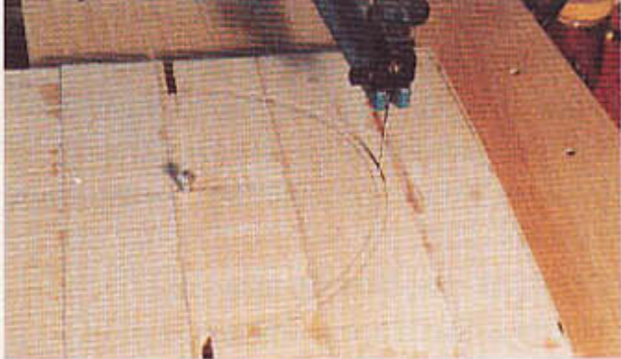
The curved door tops and valance, cut on a scroll saw with cutting jig
